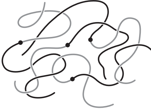
FIG. 4.3. Block copolymer melt considered in Model E. The type A blocks (dark) and type B blocks (light) are both modelled as continuous Gaussian chains. The melt is assumed to be locally incompressible.
