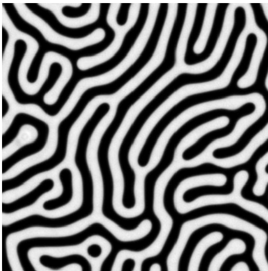
FIG. 5.20. Segment density configuration for an incompressible, symmetric diblock copolymer melt (Model E with b_A = b_B ). Parameters are \chi_{AB}N = 25.1 , f = 0.5 , L = 51.2R_g , and M = 512^2 . Figure courtesy of A. Bosse.
