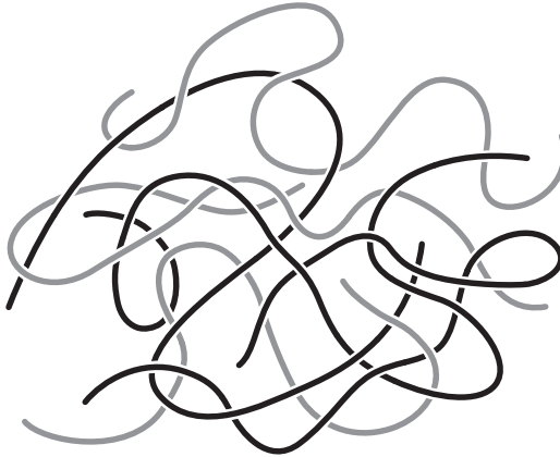
FIG. 4.2. Binary blend of homopolymers considered in Models C and D. The type A homopolymers (dark) and type B homopolymers (light) are both modelled as continuous Gaussian chains. The melt is assumed to be locally incompressible or compressible, respectively, in Models C and D.
