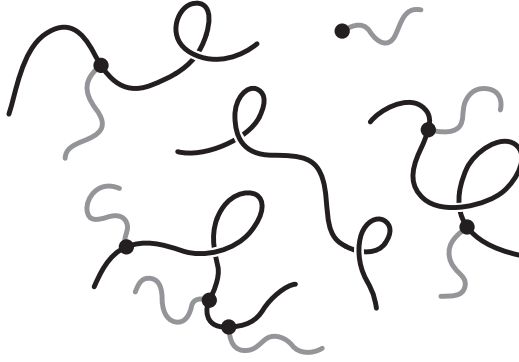
FIG. 4.6. Products of reactive coupling of A homopolymer containing uniformly placed reactive functional groups (dark) with end-functional B homopolymer (light). The resulting alloy contains graft copolymers with varying number and placement of B grafts, along with unreacted A and B homopolymer.
