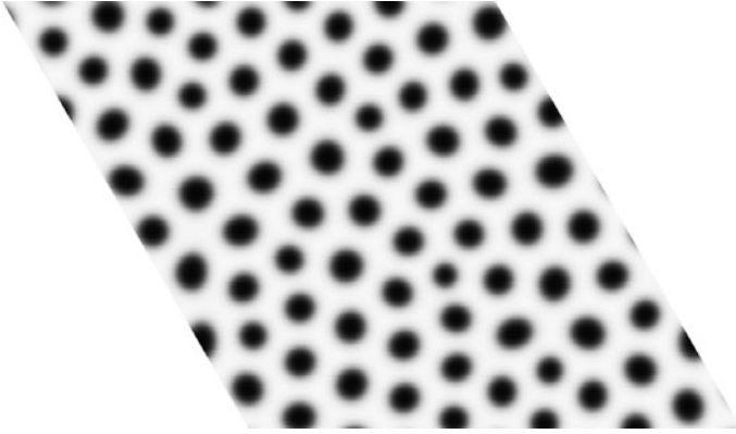
FIG. 5.10. Segment density configuration (A segments dark, B segments light) for an incompressible diblock copolymer melt (Model E with b_A = b_B ) resulting from a large-cell SCFT calculation started from random initial conditions. Parameters are \chi_{AB}N = 20.0 , f = 0.3 , L = 32R_g , and M = 512^2 . Figure courtesy of E. Cochran.
